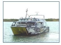
Owners Designer LOA Draft Engines Cruise Speed Whalewatch Kaikoura NZ Teknicraft Design Limited 17.7m .7m 2 x MTU 2000 M70 8V Diesel 36 Knots
